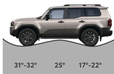
Approach, ramp break-over and departure angles
