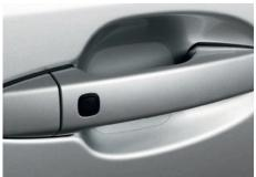
DOOR HANDLE PROTECTION FILM The door handle protection film is a tough transparent self-adhesive film that helps protect door paintwork against those small scrapes and scratches.
