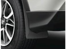
FRONT & REAR MUD GUARDS Designed to minimise water, mud and stones spraying onto your car's body.
