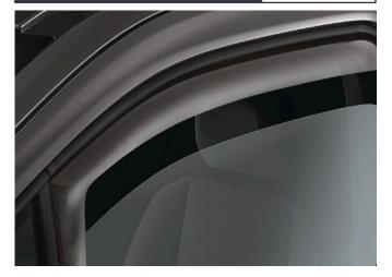
Wind deflectors are ideal if you like to drive with the windows open. They are custom designed to match the aerodynamic contours of your vehicle and work by diverting air flow to ensure that you and your passengers are not troubled by excessive wind movement and noise.
