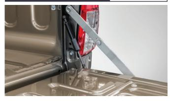
Tailgate struts are essential for the suspension of your tailgate. The strut helps facilitate closing the tailgate by assisting in pulling it upwards once you start to push/pull it upwards.
