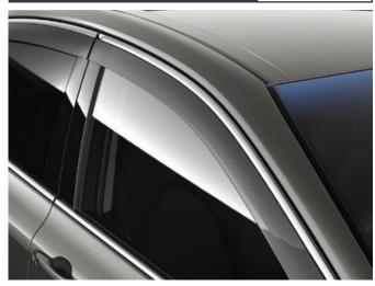
Wind deflectors are ideal if you like to drive with the windows open. They are custom designed to match the aerodynamic contours of your vehicle and work by diverting airflow to ensure that you and your passengers are not troubled by excessive wind movement and noise. Standard transparent wind deflectors available.
