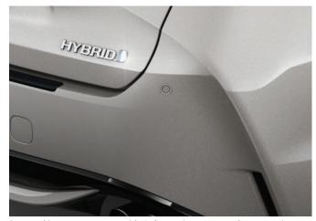
Rear parking sensor system with 4 ultrasonic sensors and an acoustic warning.
