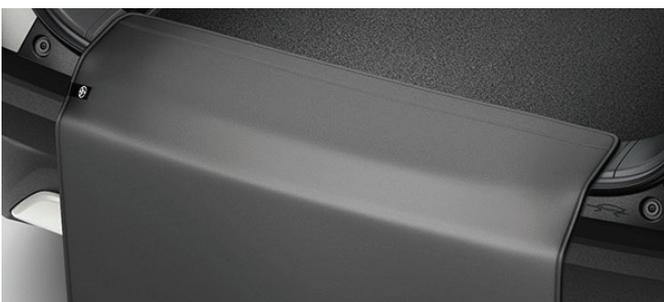
The rear bumper protection apron is fixed to the trunk deck with velcro. It protects the rear bumper when unfolded.
