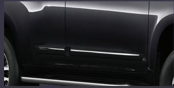
Side mouldings provide your vehicle with an extra layer of protection to help guard the side panels against minor bumps and scraps.
