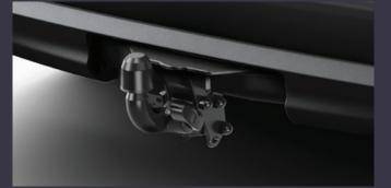
The towing hitch gives you ideal capacity to tow a trailer. It is designed for the Toyota Corolla Touring Sports and has a tough anti-corrosion surface treatment.
