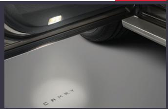
Door lamp illuminates the ground when the door is opened. CAMRY is projected on the floor.
