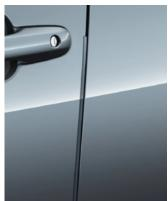
DOOR EDGE PROTECTION FILM The door edge protection film is tough transparent self-adhesive film that helps protect door paintwork against those small scrapes and scratches.
