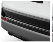
REAR BUMPER PROTECTION PLATE Designed to protect the rear bumper paintwork against scratching when sliding heavy or awkward loads into the boot. It is also particularly effective for guarding the paintwork of the boot area.
